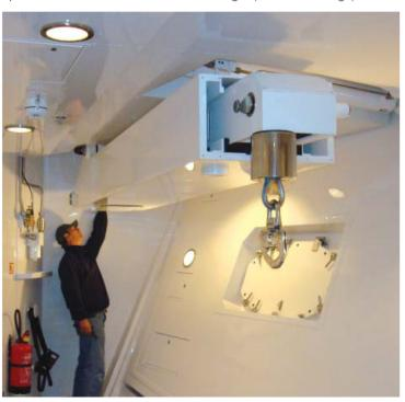
The boat booms telescope 3 metres from the side of the vacht from LR approved watertight housings. Into the final section of the boat boom we installed a specialised hydraulic linear winch system that provided a fairlead to the tender. The hydraulic circuit prevents the booms from being retracted into the yacht while the line is out of the boom. These booms are manufactured from 316-L stainless steel, and like the cranes are mirror-polished.
