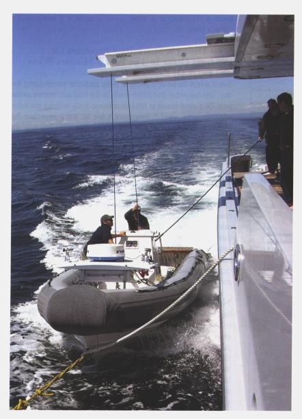
hoisting lines are released and then the tow-line is released using a load-release hook. Retrieval is done in the reverse manor; the tender will run up to the towing boom and hook-up, then attach the hoisting lines.
