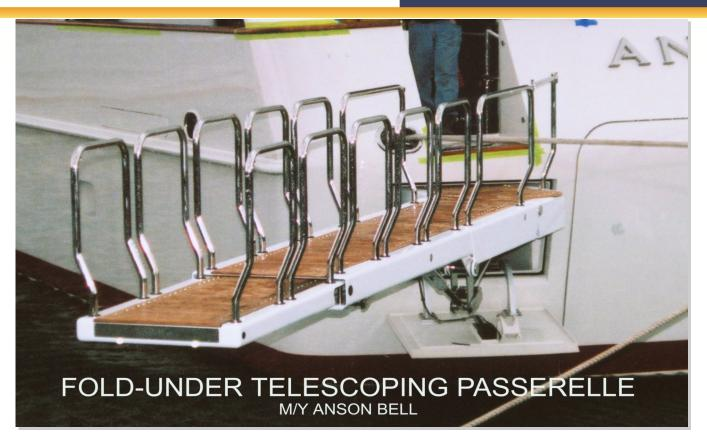
The fold-under passerelle provides a unique solution for vessel designs with limited stowage space or requirements for enhanced deployment length. The folding design provides the greatest efficiency in the stowed:deployed ratio. This ratio is further enhanced when the folding plank section includes an additional telescoping plank section. The passerelle folds in a "stacked" fashion when stowed.
