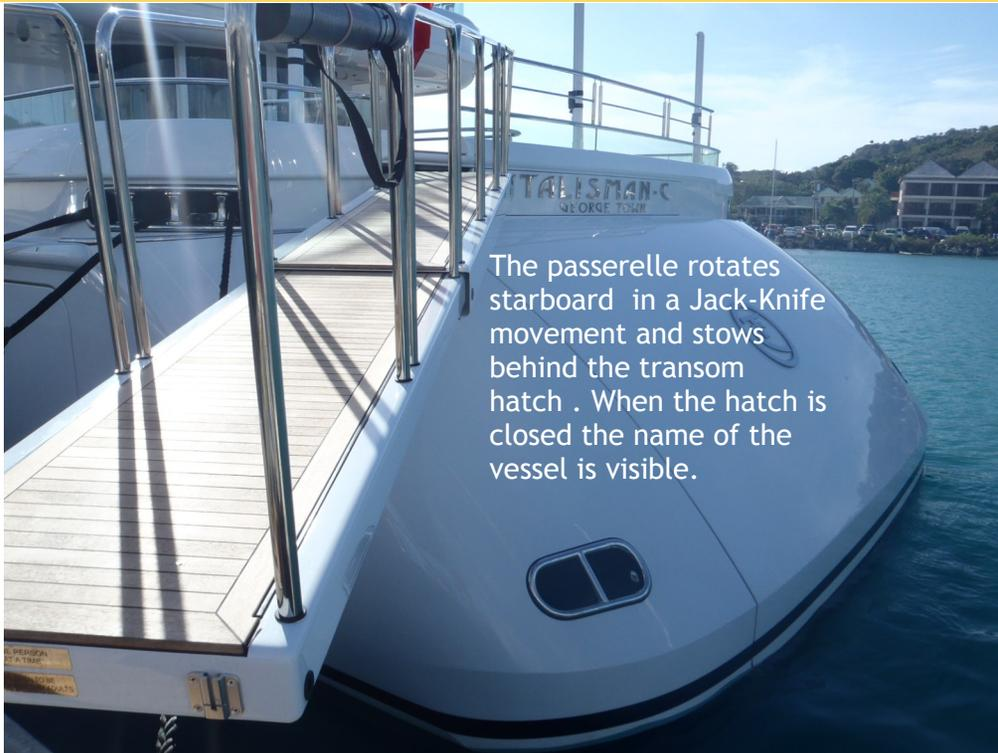
The passerelle rotates starboard in a Jack-Knife movement and stows behind the transom hatch. When the hatch is closed the name of the vessel is visible.
