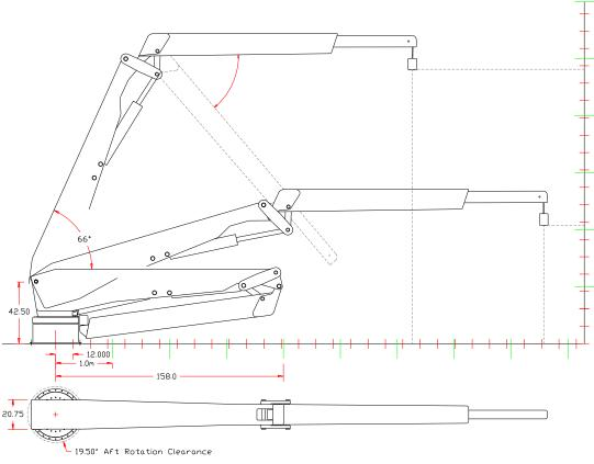
Cylindrical style pedestal bases are required and will be configured for specific applications. Floating-Flange standpipe mounting is available for GRP constructed vessels. Standpipe diameters will vary depending on the actual moment capacity of the crane.
