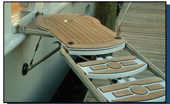
Top: Rotation Platform; allows the stairway to rotate 160°.
